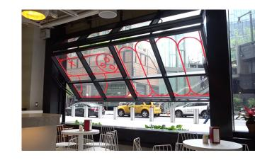
sidewalk traffic while flooding the space with natural light. With a push of a button, the impressive 12′ 10″ x 7′ 8″ motorized partition quietly folds upward along a horizontal hinge line creating an awning effect.
